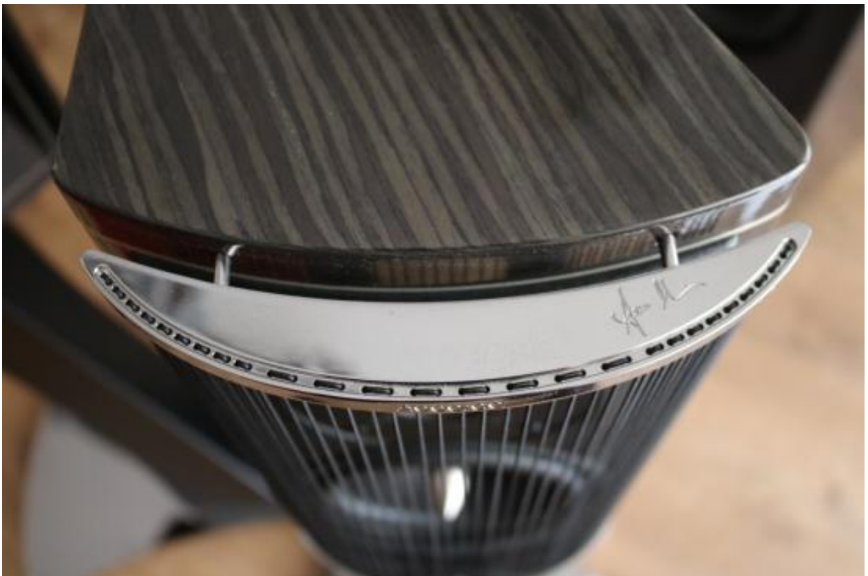
Above: the grill can easily be removed by gently pulling off the top and bottom parts.
